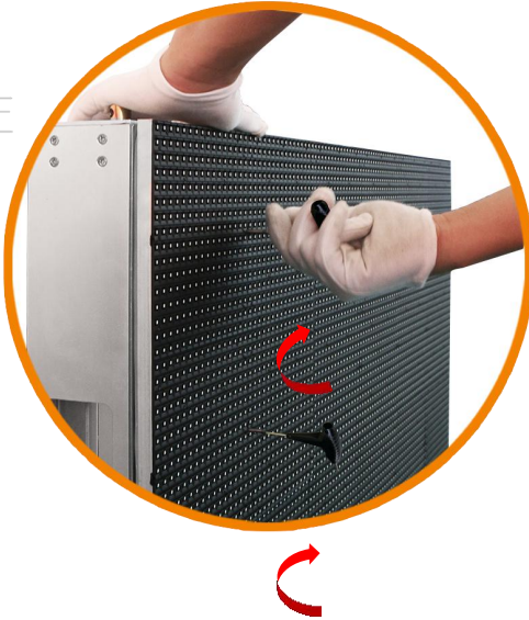
Insert the upper and lower unlocking tools into the front maintenance hole, and rotate 90 degrees to the left to unlock.
