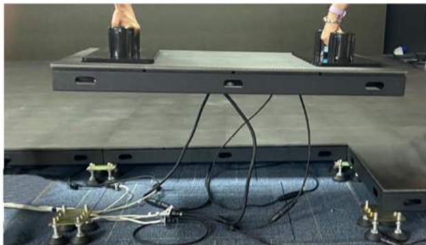
Vacuum module maintenance
